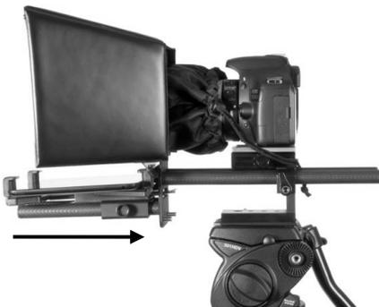
20. Put the configured tablet into the mounting bracket and ensure it is held securely by adjusting the size of the bracket holders for a snug fit and locking them in place. Use the locking lever on the bottom of **item H**.
