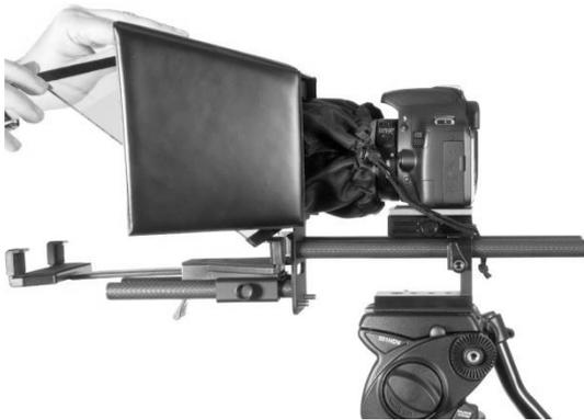
18. Now insert the Mirror glass, **Item J**. There are Velcro edges on the glass, marry these edges to the Ridge/Groove on **Item D (bottom)** and Velcro on **Item I** (top) so it is secure. The shortest edge of the Mirror glass should be at the bottom.
