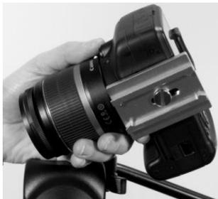
4. Attach the camera plate from **Item A** to the base of the DSLR camera. Now slide the camera and plate into position on top of **Item A**.
