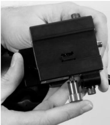
3. Remove the sliding camera plate from the top of **Item A**. Do this by pressing in the side screw on **Item A** once it has been unscrewed half way.
