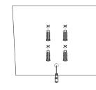
Insert the plastic wall anchors into the 6 mm diameter holes.
