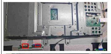
Remove the two screws on the mainframe and then disconnect the FFC cables
