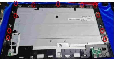
Remove the screws on the middle frame
