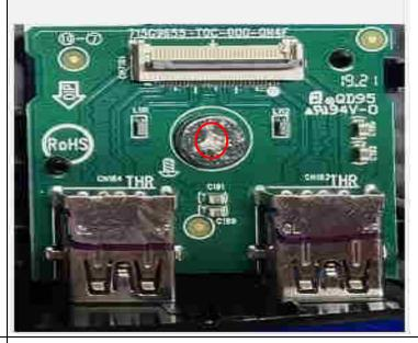
Remove the screw on the usb board
