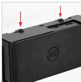
Security screws to prevent easy removal of Pod device.
