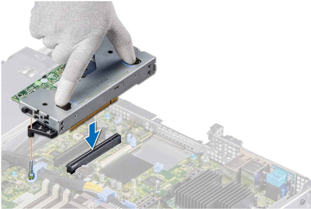
Figure 56. Installing the low profile left riser
