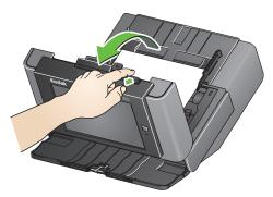
2. Remove any jammed document(s), close the Scan Station cover and resume scanning.
