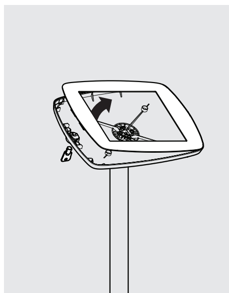
6 Unlock & remove the Faceplate from the Bouncepad Case.
