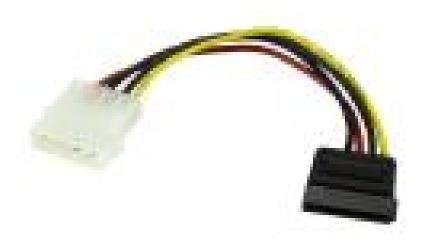
This 6in 4 Pin LP4to SATA power adapter cable features one 4 Pin LP4 male connector and one female SATA power connector, allowing you to power a Serial ATA hard drive from a conventional LP4 connection, eliminating the need to upgrade the computer power supply for compatibility with the SATA hard drive.
