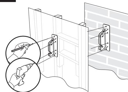
Minimum Installation Requirements when mounted to wood studs:  $\frac{1}{4}'' \times 1\frac{1}{2}''$  (M6 x 38 mm) lag screw
