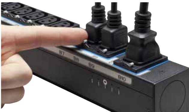
Figure 3. IEC outlet grips provide plug retention and eliminate the need for intrusive cable management that often blocks airflow and decreases serviceability.
