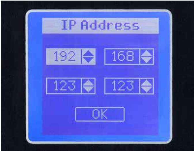
Figure 2. An advanced pixel LCD screen with pull-down interactive menu options on a rack PDU.
