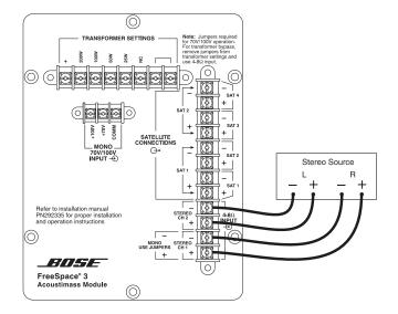
Please note: In setting up this operation, the following situation may occur: During system testing, while the source drives one channel only (shown right), a reduced output from the other channel is audible.
