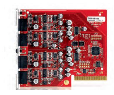
The Tesira® SOC-4 is a modular analog output card for use with Tesira SERVER or SERVER-IO devices. Each SOC-4 provides 4 channels of mic or line level audio output. The outputs are electrically balanced and provided on plug-in barrier strip connectors. Software control of each output includes mute, level, signal invert and full-scale output reference.
