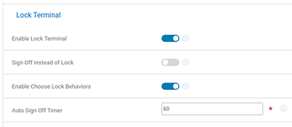
Figure 2. Lock Terminal in Wyse Management Suite
