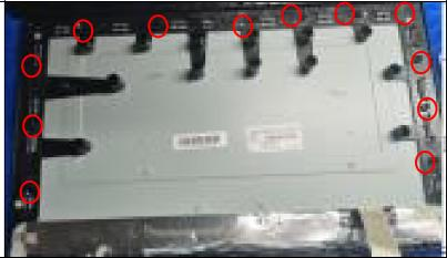
Remove the screws on the middle frame
