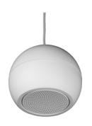
The EN-SPH5T16-W is a compact **5.25**" sphere loudspeaker with ABS housing (UI94 HB) (RAL 9010 equivalent), equipped with a high efficiency full range speaker and a multi tap 100 volt transformer, all certified according EN 54-24.
