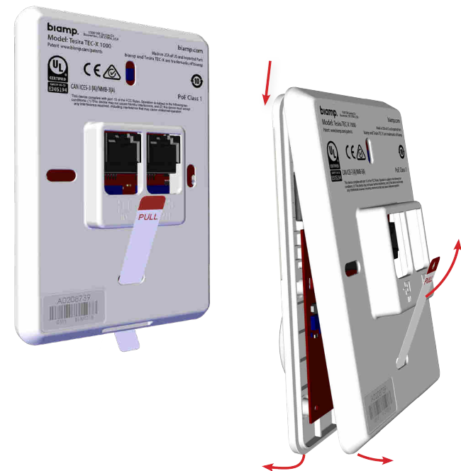
Figure 2. Separate face plate from back plate.
