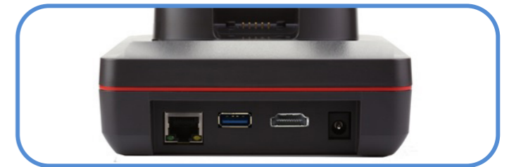
Ethernet USB A HDMI POWER Rear View
