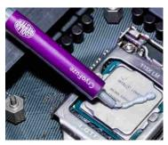
**CryoFuze Thermal Paste**
