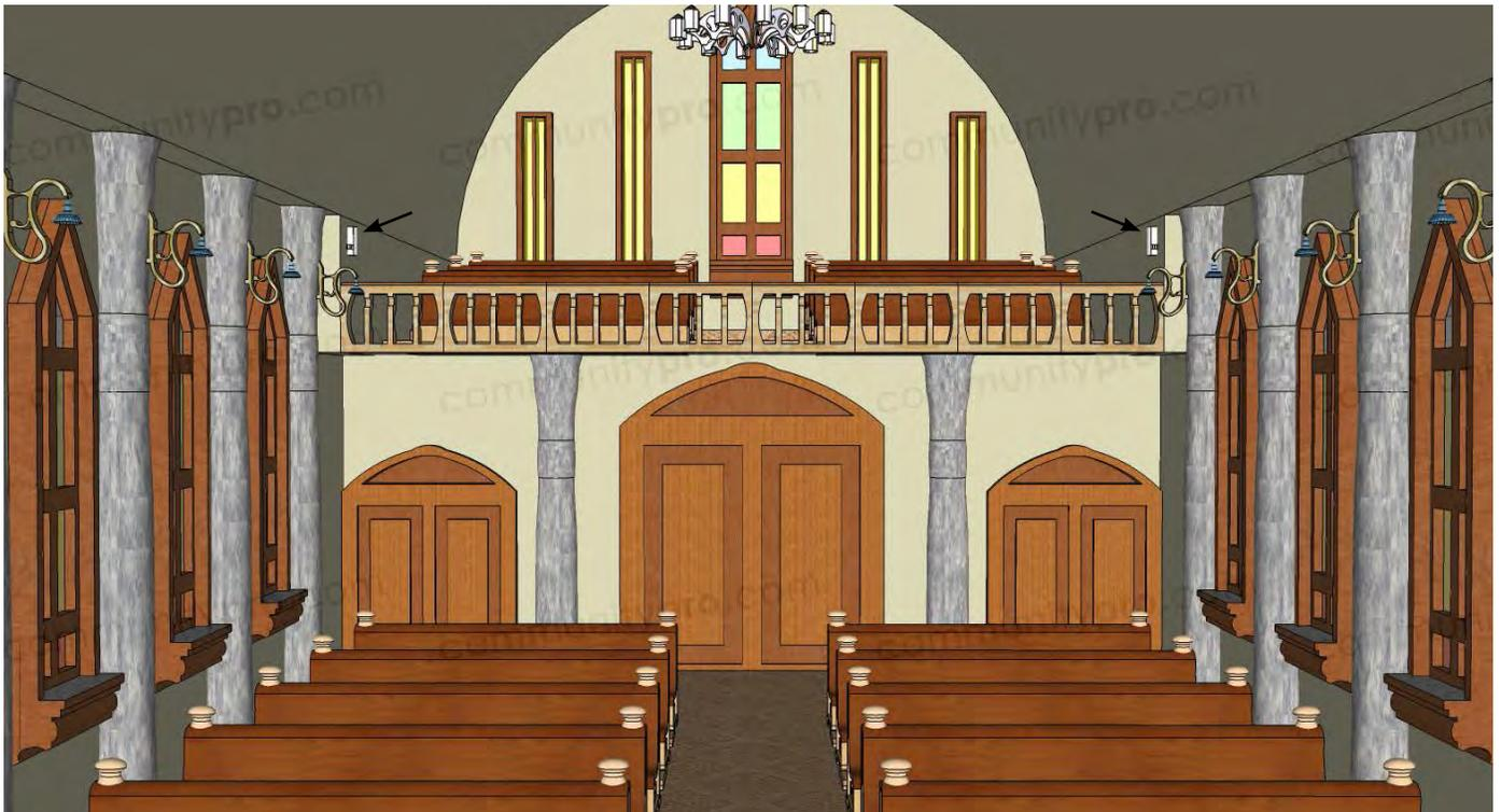
The above view shows the two ENT203s that cover the balcony, one on either side. Below is a 3D rendering depicting highly uniform coverage throughout the front, sides, and rear.
