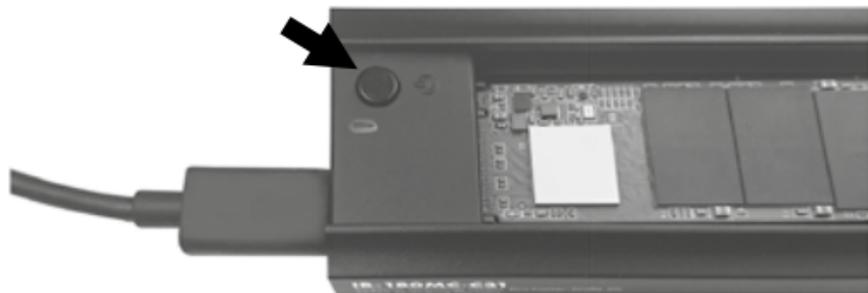
8. To deinstall the M.2 SSD please press the ON/OFF button again to power off the IB-180MC-C31 (power LED red).
