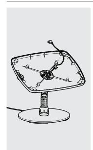
Feed the tablet cable through the Bouncepad Case & mounting arm
