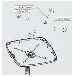
Install the Tablet Setup Kit. Each kit is speci c per tablet device and Bouncepad Case.
