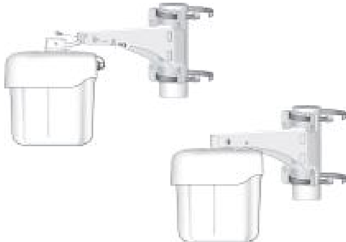
Figure 6 Attaching the AP to the Mounting Bracket
