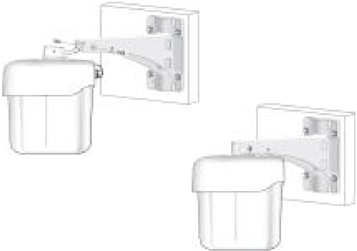
Figure 2 Attaching the AP to the Mounting Bracket
