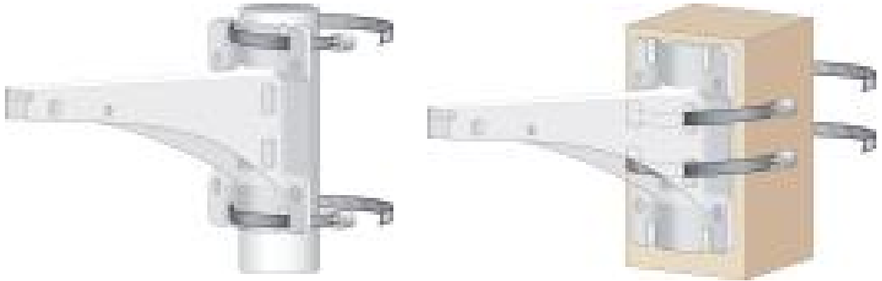
Figure 5 Attaching the Mounting Bracket to a Vertical Pole
