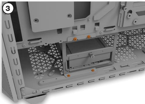
**EN** INSTALLATION OF DRIVES INTO THE SINGLE HDD CAGE FOR LARGER PSUs
