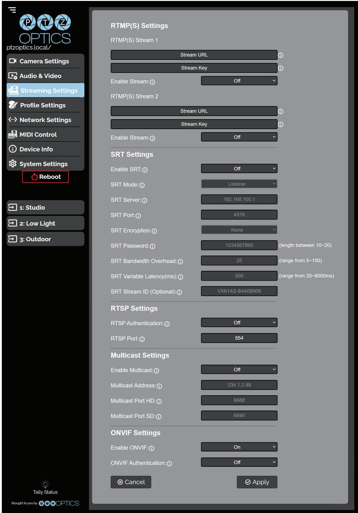
The screenshot shows the PTZ OPTICS interface with the Streaming Settings page open. The left sidebar contains navigation options: Camera Settings, Audio & Video, Streaming Settings (selected), Profile Settings, Network Settings, MIDI Control, Device Info, System Settings, and a Reboot button. Below the sidebar are three scene buttons: 1: Studio, 2: Low Light, and 3: Outdoor. The main content area is divided into several sections:
