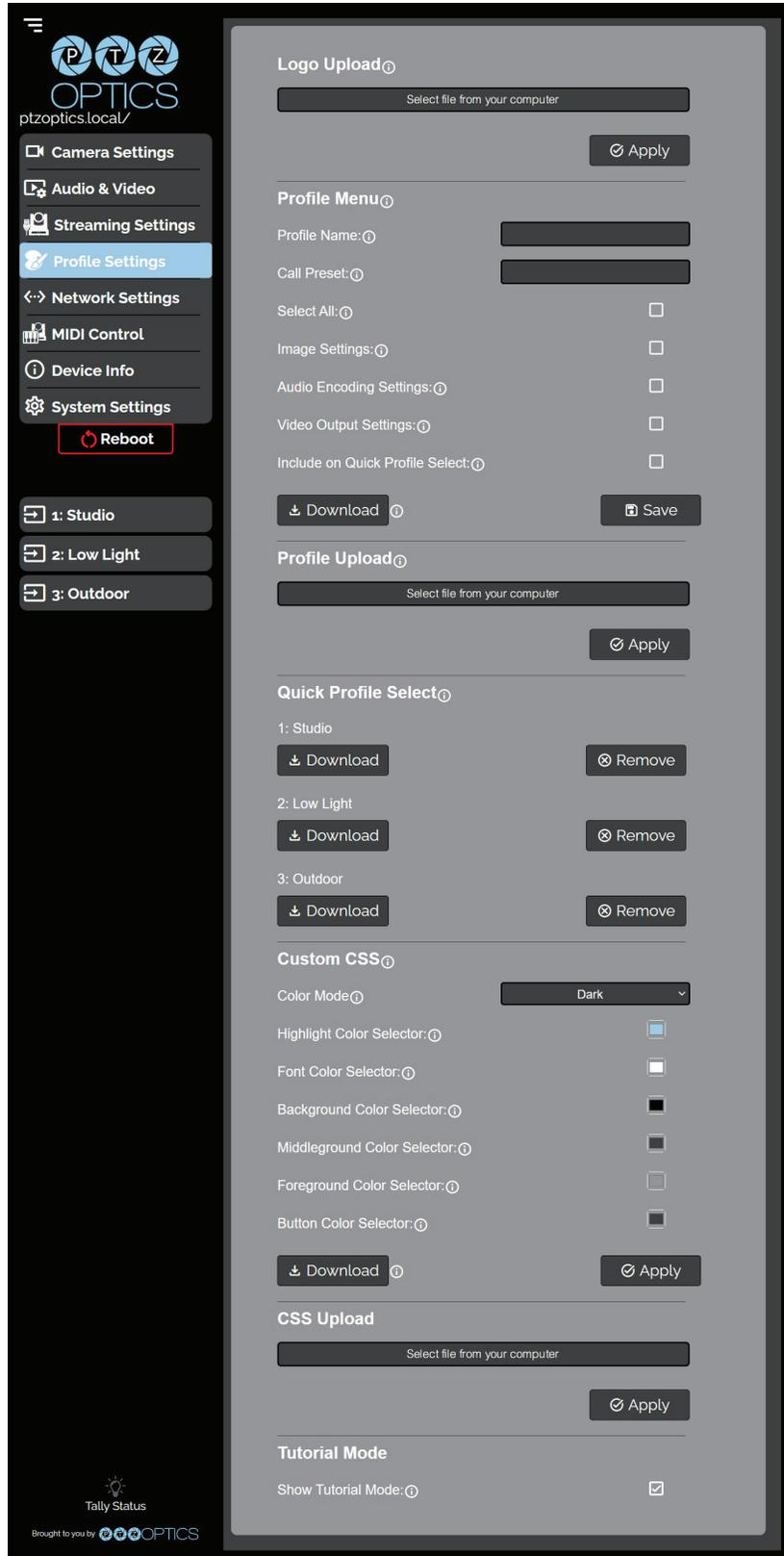
The screenshot shows the PTZ OPTICS web interface for Profile Settings. On the left is a dark sidebar with navigation options: Camera Settings, Audio & Video, Streaming Settings, Profile Settings (highlighted), Network Settings, MIDI Control, Device Info, System Settings, and a Reboot button. Below these are three profile buttons: 1: Studio, 2: Low Light, and 3: Outdoor. The main content area is divided into several sections:
