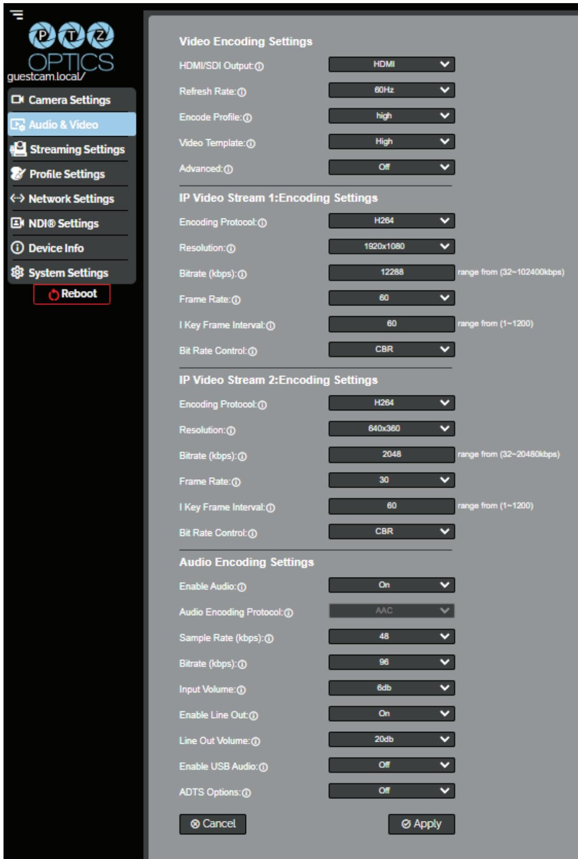
The screenshot shows the 'Audio & Video' settings page in the PTZ Optics web interface. The left sidebar contains navigation options: Camera Settings, Audio & Video (selected), Streaming Settings, Profile Settings, Network Settings, NDI® Settings, Device Info, and System Settings. A 'Reboot' button is also present. The main content area is divided into three sections:
