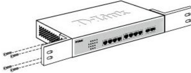
Figure 3-2 Attach the mounting brackets to the switch
