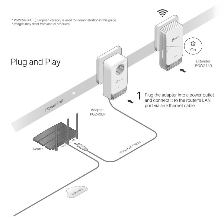
Plug the extender into a power outlet on the same electrical circuit. Wait until the extender's Powerline LED turns solid green.
