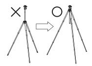
For best results and to avoid unnecessary camera vibrations, try to keep the center column height to a minimum if possible. Also use the larger legs first when extending the legs.
