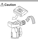
Fix the shoe lock knob firmly after inserting the quick release shoe to the platform.
