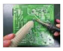
S18-5 Lift the bulk cap. up and away from the PCB.
