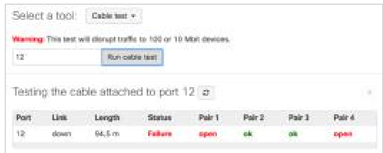
Remote cable test in the Meraki Dashboard
