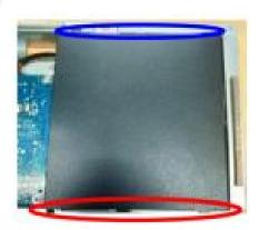
Unlock 10 PCBA screws to disassemble I/F BD, SPS BD and LED Driver BD from Main SHD
