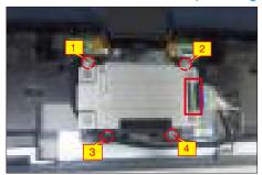
Use a Philips-head screwdriver to remove 4pcs screws for unlocking the bracket chassis with the panel, then disconnect the Mic cable away from the connector of the main board.
