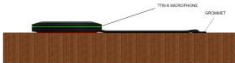
Figure 6 Tabletop with Grommet Installation Option
