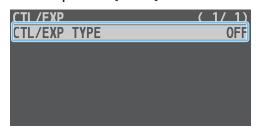
Use the [VALUE] knob to specify "EXP" (expression pedal) as the device that's connected to the CTL/EXP jack, and then press the [VALUE] knob.
