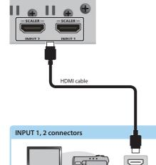
These input video. Connect these to a video camera, video device such as a BD player, or a computer that is equipped with an HDMI output connector.
