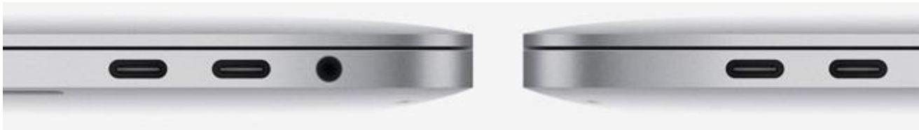
Figure 1: Two or four USB-C type connectors indicate a MacBook Pro or MacBook Air with Thunderbolt ports.
