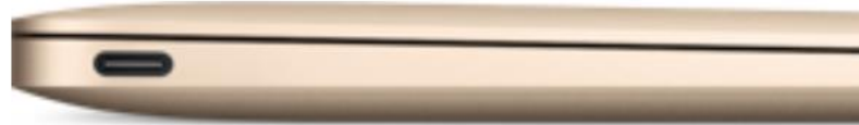
Figure 2: A single USB-C type connector indicates a MacBook with a USB 3 port. This is not a Thunderbolt port.
