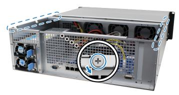
**b** Put back and fasten the screw you removed in step 2.
