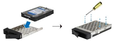
• For 2.5" drives: Place the drive in the drive tray. Turn the tray upside down and tighten screws into the four spots indicated below to secure the drive in place.
