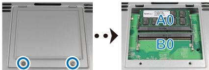
**Note:** When you remove the cover, sensitive internal components are exposed. Avoid touching anything other than the memory assembly when removing or adding memory.
