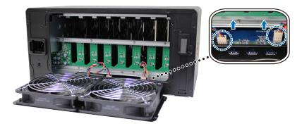
${\bf c}\,$  Remove the screws that secure the fan from the fan case.
