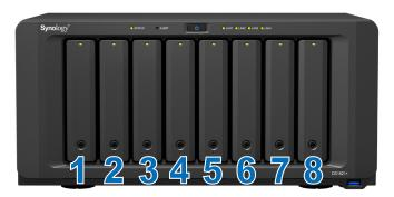
**Note:** If you plan to create a RAID volume, we recommend installing drives of identical size to make the best use of drive capacity.
