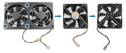
**d** Remove the screws that secure the fan guard from the malfunctioning fan.
