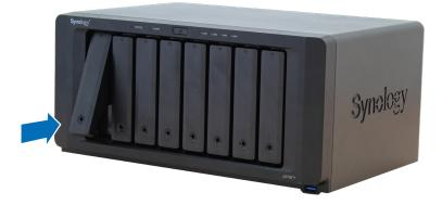
2 Pull out the hard drive tray handle as shown below to remove the hard drive tray.
