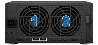
**3** Remove the four screws that secure the fan panel.
