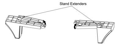
4. Stabilize the stand extenders by screwing M4 screws from the hooks to the tower stand pieces.
