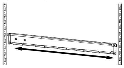
4. Screw a M6 screw into each of the bottom holes to fix the rail slider in place for both ends of the rail, and for both rail sliders (a total of 4 M6 screws are used here).
