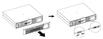
3. Remove the cover of the External Battery Connection Port using a screwdriver.
