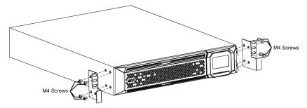
7. Fit the UPS onto the rack rails and stabilize the mounting kit (M6 screws) onto the rack as shown:
