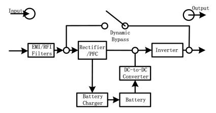
The UPS is composed of a mains input, EMI/RFI filters, a rectifier/PFC, inverter, a battery charger, a DC-to-DC converter, a battery package, a dynamic bypass and an UPS output.
