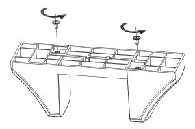
2. Bend the tower stand as shown in the diagram below:
