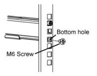
5. Insert the M6 nuts onto the support columns as show below:
