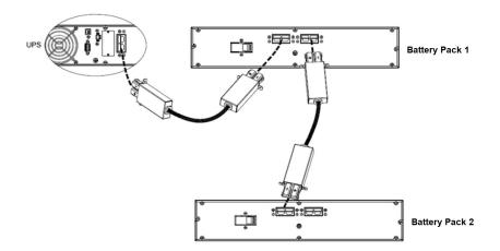
5. Stabilize the connectors to the unit and the battery pack(s) using screws. An example is shown below:
