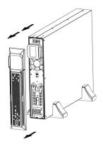
3. Turn the LCD panel such that the buttons are below the LCD screen.
