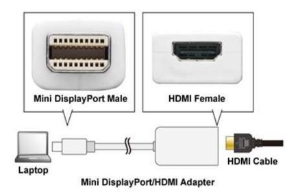
Mini DisplayPort Male to HDMI adapter for connection of any miniDisplay port devices such as Apple Macbooks, Microsoft Surface, Dell Laptop, or any other device with a Mini DisplayPort output. This little device lets you connect your device to any HDMI monitor / projector with ease. Mini Display Port is also known as MiniDP. These MiniDP ports can be found on many Macs, Laptops and Tablets plus some graphics cards. Please check your device manual for compatibility information.
