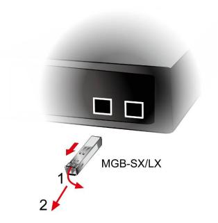
Figure 2-1-8 How to Pull Out the SFP Transceiver
