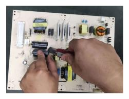
S25-2 Ensure cutting path within the glue, don't touch bulk cap. or PCB.
