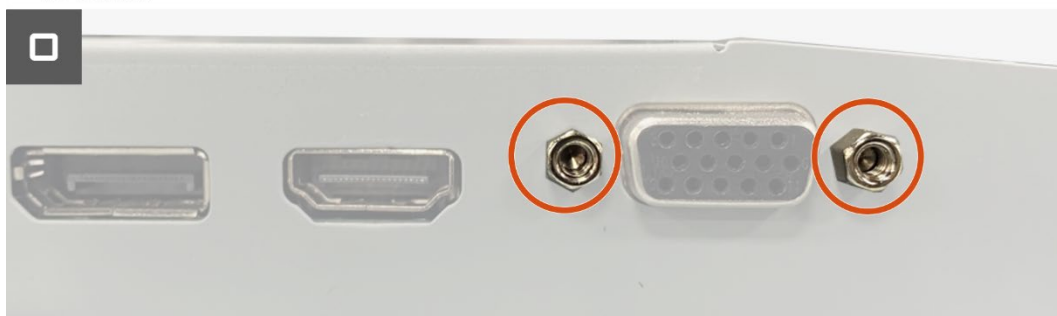
Figure 32. Installing the interface board
