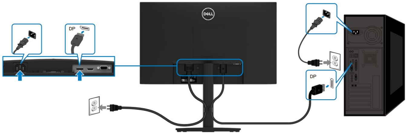
Figure 7. Connecting DP cable
