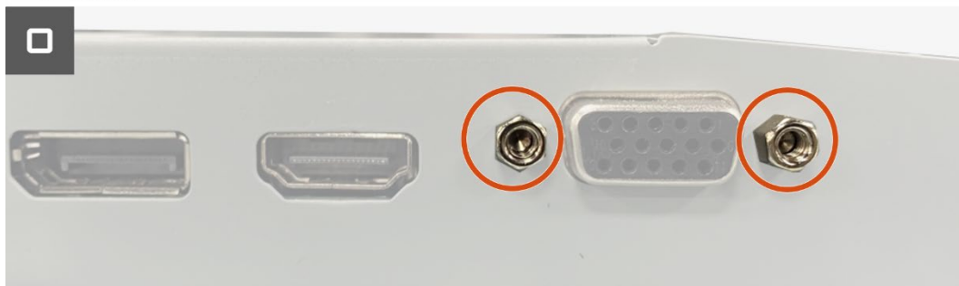
Figure 32. Installing the interface board
