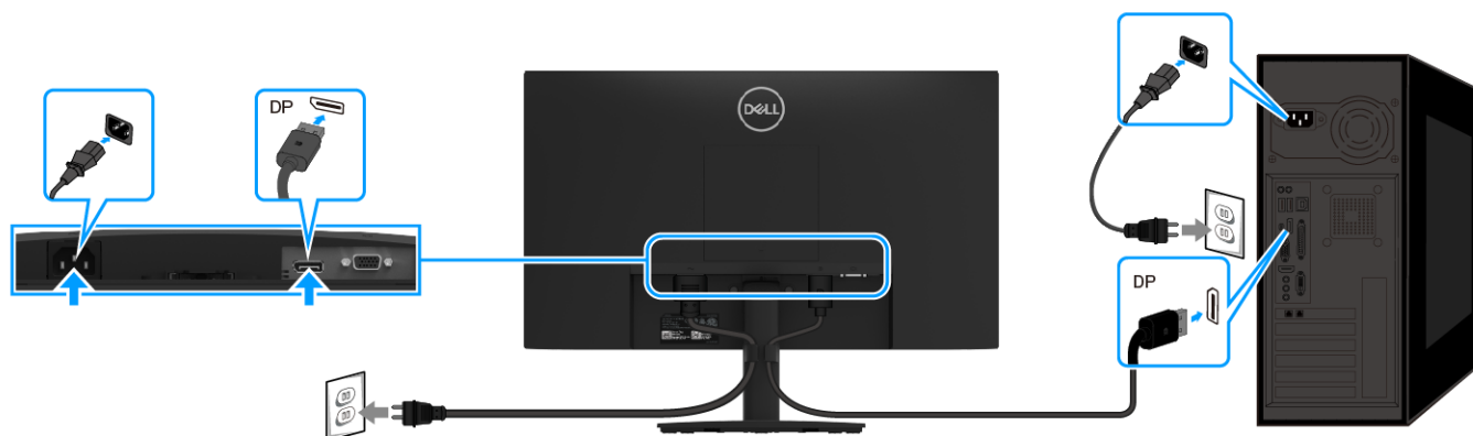
Figure 7. Connecting DP cable
