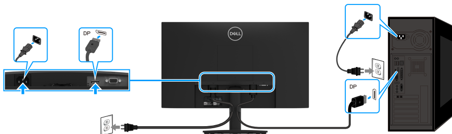
Figure 15. Connecting DP cable
