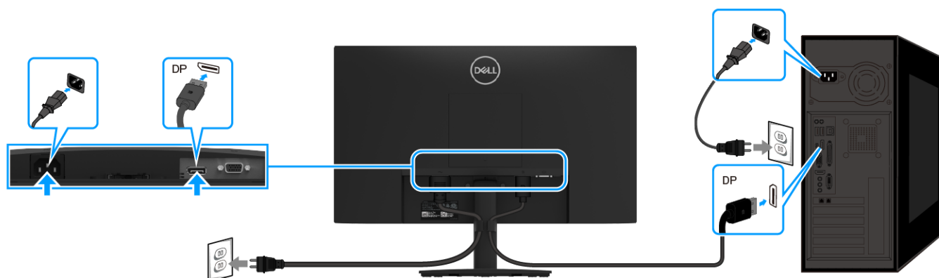
Figure 7. Connecting DP cable
