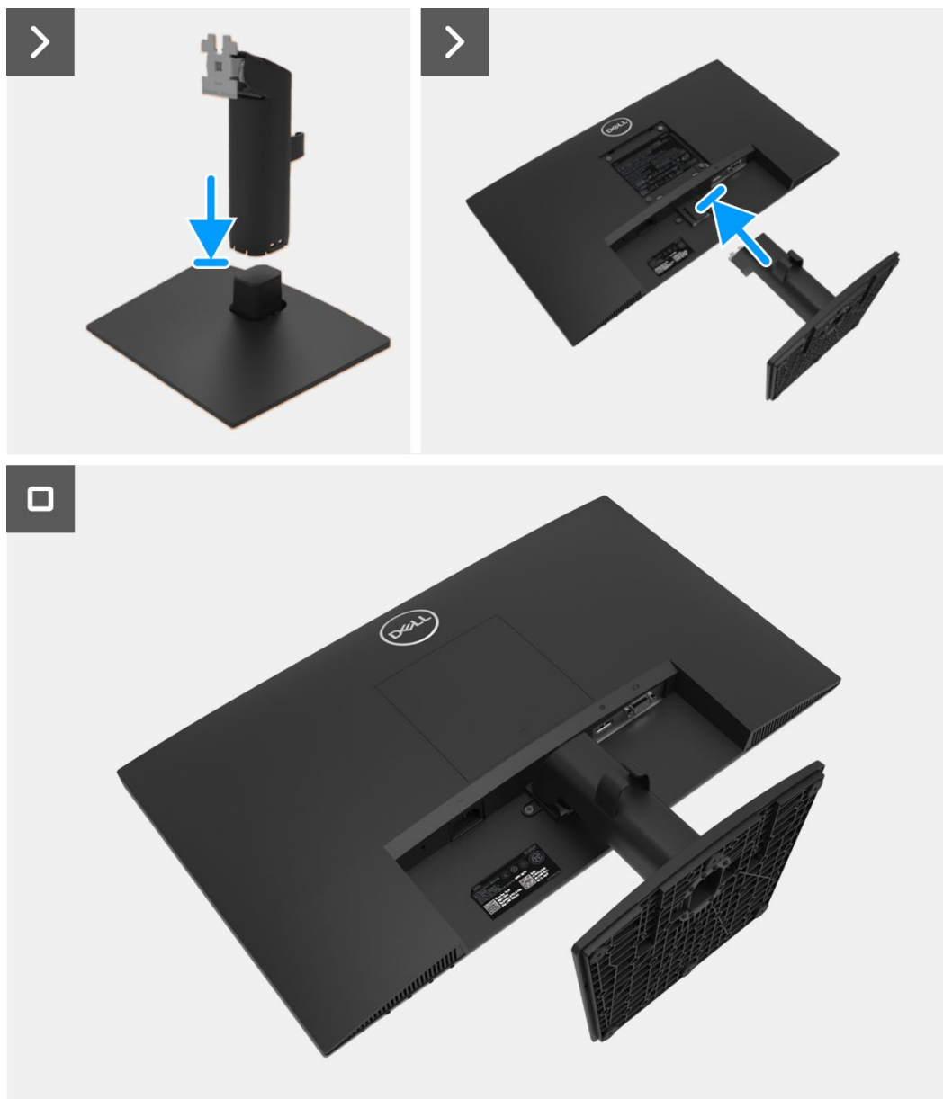
Figure 9. Installing the stand
