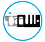
2. Route up to three **Peripheral Cables** through the **Cable Channels**, then slide the **Collector Buckle** inward.
