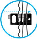
Secure the Collector Buckle in place by routing either the shackle of a Lock or a Tether Cable through the Lock Hole.
