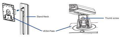
② Install the Stand-Neck to the Stand-Base and then tighten the 'thumb screw' to secure them.
