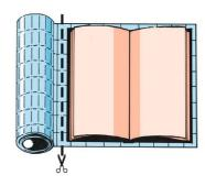
3. Then peel back approx. 10 cm of the backing paper or backing film (filmolux® soft) and align the film on three sides, position on the book cover and press the edge of the film down.
